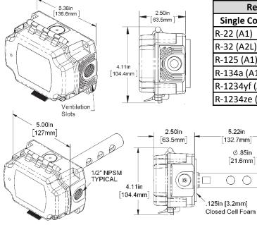
Output Voltage: 0 to 4.8 VDC Ambient Temp: 32 to 140°F (0 to 60°C) Sensor Element Life: 2 Years Typical Warranty: 2 Years
